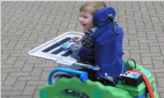
Figure 3: Bugzi – a powered indoor wheelchair for children aged 0 – 5
